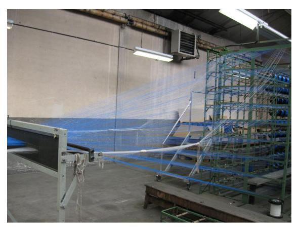
The operation of winding warp yarns under equal tension, arranged both parallel to each other and in a certain order.
