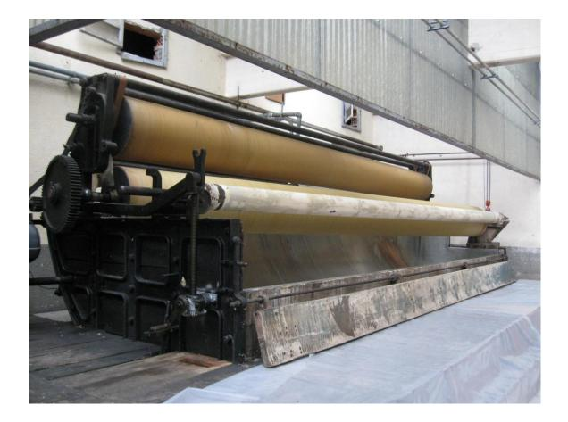
This operation follows that of the fulling mill, and consists of washing the woolen felt (degreasing, removing fibre residue...) before drying.
