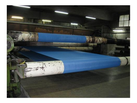
This operation gives drying wires dimensional stability (length, width, thread count, porosity) and strengthens the needled fibres onto the base of wet section felts.
