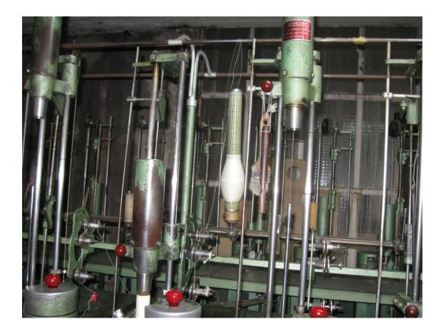
This process is the preparation of the weft threads, and is completed in the form of pirns/quills (cylindrical or slightly tapered support on which yarn is wound)
